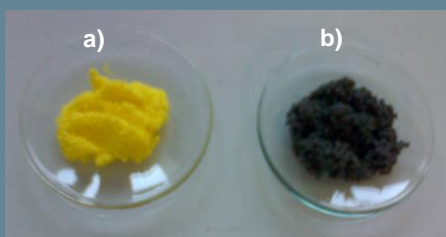
Figure 1 : a) bulk AMP-PAN Resin, b) bulk KNiFC-PAN Resin
