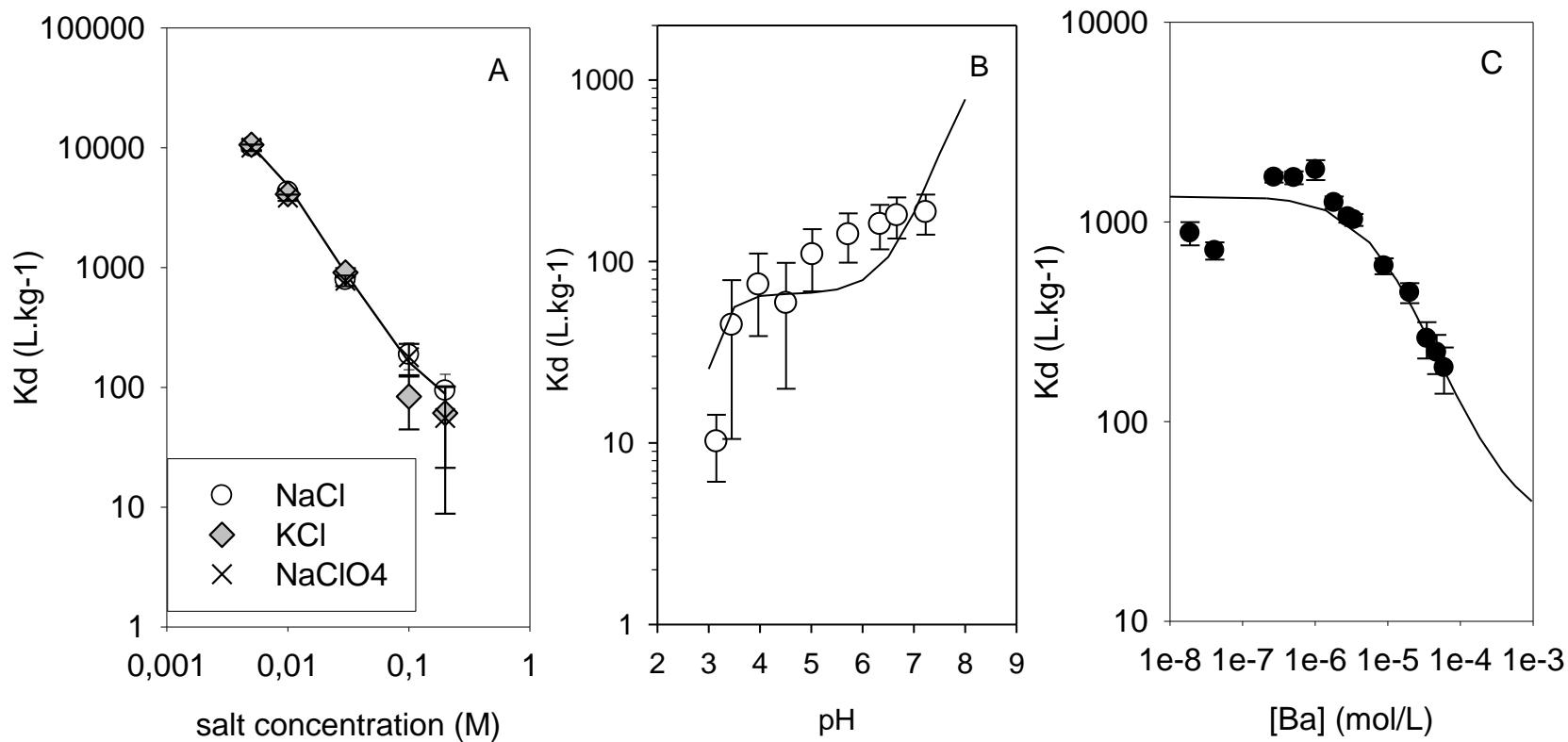
Sorption of Ra and Ba on GR in salty waters; m/V of 1 g.L<sup>-1</sup>. (A) Effect of the type of salt and its concentration on Ra adsorption; pH=7.0 ± 0.1;. (B) Effect of the pH on Ra adsorption in 0.1M NaCl. (C) Sorption isotherm in concentration for Ba in the presence of 9.2 10<sup>-3</sup> M of NaCl.
