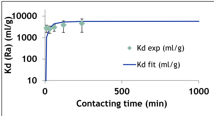
→ > 80% of  $^{226}\text{Ra}^{2+}$  adsorbed after 10 min of contact.: **Rapid kinetics**
