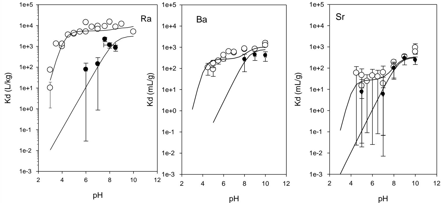
Adsorption of  $\text{Ra}^{2+}$ ,  $\text{Ba}^{2+}$  and  $\text{Sr}^{2+}$  ions with grafted (black symbols) or ungrafted (white symbols) silica as a function of pH. The m/V ratio is fixed at 2.5 g.L
