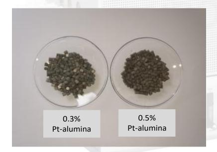
More robust supply of material. 0.5% Pt-alumina is being phased out. Tested with <sup>3</sup>H-thymidine spiked milk.
