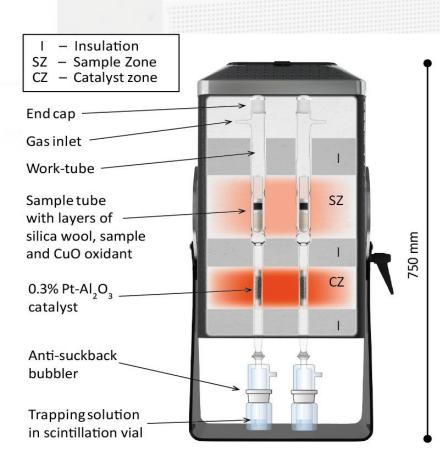
Samples loaded at 600°C then heated to 900°C.
